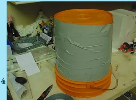
This is what the taped bucket will look like when completed the adhesive side ( sticky side will be out the non sticky side will be against the bucket
