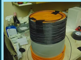
This is progressing as the wire is being wrapped or coiled or turned on the bucket you can see it is pretty uniform with some slight gaps -again do not worry about that but do try to get them as close as you can so you have a uniform or a wiring that is pretty good
