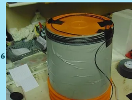
AS you can see you just start to "coil" or wrap the bucket and you try to keep it as tight as you can to the proceeding wrapping if not just go back and re thread the wire around the bucket- it will work if there is a little space so do not be concerned to a oint of frustration- your not running a race and your not punching a clock your building a means to assist you in your health against the nano afflictions
