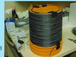
This is the Bucket completely wired or coiled or wrapped all the way and you just tape the ends at the other end when you finish so that it does not unravel and you cut another 2 ft of wire from the spool or container you are getting your wire so you have about 2 ft on each end of the bucket
